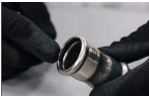
Controllo O-ring / Checking the sealing ring
